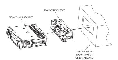
TYPICAL FRONT-LOAD DIN MOUNTING METHOD
