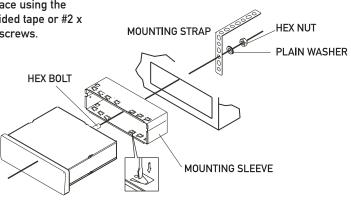
TYPICAL FRONT-LOAD DIN MOUNTING METHOD
