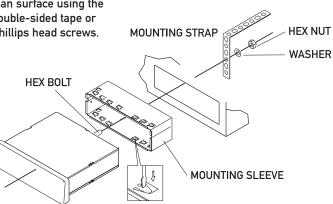
TYPICAL FRONT-LOAD DIN MOUNTING METHOD
