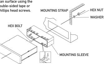
TYPICAL FRONT-LOAD DIN MOUNTING METHOD
