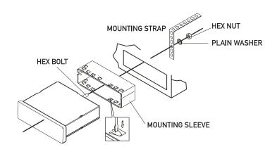
TYPICAL FRONT-LOAD DIN MOUNTING METHOD
