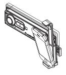
Line up the dock connector on the iPod/iPhone device with the connector located on the bottom of the dock.
