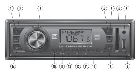
Power / Source Tune / Track Down 1 9 2 10) Mute / Loud Preset 6 3) 11) Volume Preset 5 / Folder Up 4 (12) Tune / Track Up Preset 4 / Folder Down 5) Band / Auto Station Store (13) Preset 3 / Play / Pause 6 SD Card Slot Preset 2 / Random 14 7 Auxiliary Input (15) Preset 1 / Repeat 8 USB Port Audio / EQ 16
