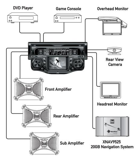
The diagram above illustrates the connection capabilities of the XDVD8130. Two separate Audio/Video inputs allow the connection of a DVD player or game console. The video output provides signal to external monitors - such as an overhead or headrest type. A rear view camera can be connected to provide assistance when backing up your vehicle. Visit your local DUAL dealer for more details.
