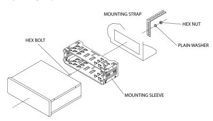
TYPICAL FRONT-LOAD DIN MOUNTING METHOD
