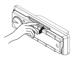
To open the XML8110 and use the iPod dock, pull outward from the top of the front panel.
