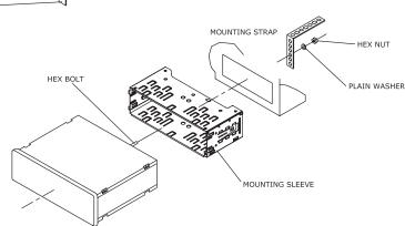
TYPICAL FRONT-LOAD DIN MOUNTING METHOD
