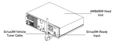
Line up the connector with the pins on the cable. It can only be inserted as shown above. Push the cable into the head unit's connector until it clicks. Attempting to insert the cable differently from shown above may cause damage to the cable or head unit.
