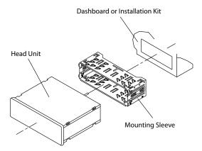
TYPICAL FRONT-LOAD DIN MOUNTING METHOD
