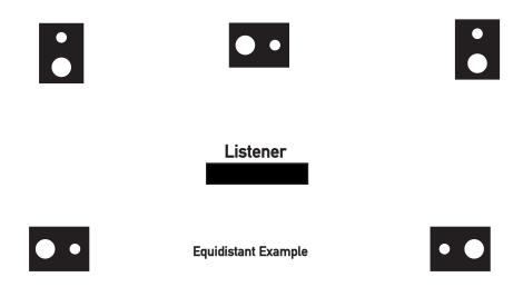
The speaker imaging decreases rapidly the further the listener is from the speakers, so an equidistant speaker arangment for multi-channel installation is desired for the best results. Try to equalize the speakers distance so the listener is basically in the middle of the sound stage.
