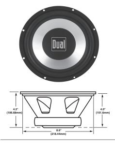
XS10 Sensitivity: 87dB Freq. Response: 30Hz-125Hz Nominal Impedance: 4 ohms Peak Power: 400 watts RMS: 150 watts Voice Coil Size: 2" Magnet Size: 24oz.
