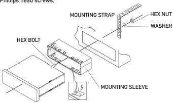
TYPICAL FRONT-LOAD DIN MOUNTING METHOD
