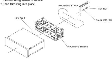
TYPICAL FRONT-LOAD DIN MOUNTING METHOD
