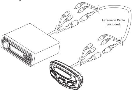
Once the remote has been mounted, connect the cables to the remote and head unit as in the diagram above. When routing the extension cable, be sure to avoid sharp objects, corners, and places where it might get pinched, as this could affect performance and cause damage to the unit.
