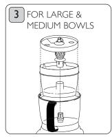
The adjustable slicing disc can only be used with the large and medium bowls. It creates any slice thickness between 0.5mm and 7.5mm.
