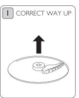
The julienne disc must be inserted with the cutting face upwards.
