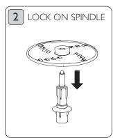
Place the reversible shredding disc on the spindle and push down firmly to locate.
