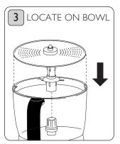
Place the spindle and grating disc assembly onto the bowl drive of large processing bowl.
