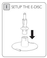
Attach the spindle onto the centre of the E-disc. Push down until you hear and feel in the large bowl. it lock into place.
