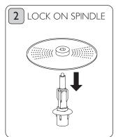
Place the reversible grating disc on the spindle and push down firmly to locate.
