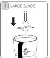
Handle blades and attachment The medium chopping blade using only the central plastic section. The large chopping blade locates directly onto the bowl drive, once the large place. bowl is locked in place.
