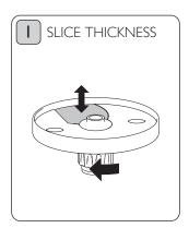
To adjust the slicing thickness, Firotate the outer spindle squanti-clockwise to make slices publicker, or clockwise to make thinner slices. NOTE: Very sharp. Hold plastic to avoid injury.
