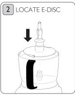
Place the E-disc assembly directly onto the bowl drive
