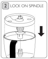
Fit the slicing disc over the spindle and press firmly into place.
