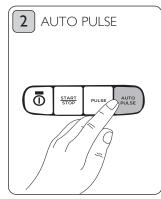
Press the 'AUTO PULSE' button to start processing. The blade will automaticaly pulse 10 times. To stop mid cycle press 'START/STOP' button.
