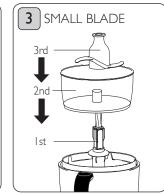
The small chopping blade needs to be used with the spindle. This must be attached to the bowl drive once the large and medium bowls are in place, and before locating the small bowl.
