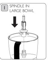
The spindle locates on to the bowl drive on the large processing bowl.
