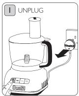
ENSURE THE PROCESSOR IS UNPLUGGED WHILST IN STORAGE, WITH THE LID UNLOCKED. THOROUGHLY CLEAN AND DRY.
