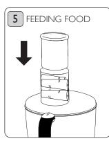
Feed items gently through the feed tube using the food pusher. Let the disc do the work. Exerting too much pressure will damage your machine. NEVER USE YOUR FINGERS!
