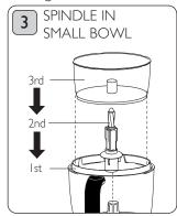
When using the small bowl with blade, place in the large bowl with medium bowl. spindle in position, then place the small bowl and small blade on the spindle.
