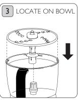
Place the spindle and shredding disc assembly onto the bowl drive of large processing bowl.
