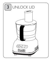
Store the bowls and lid with food pusher assembled on the processor body. Do not lock the bowl lid whilst in storage. This can damage the safety mechanism built into the bowl.
