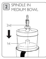
When using the medium bowl, place it in the large bowl then the spindle on the howl drive.
