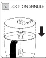
Fit the julienne disc over the spindle and press firmly into place.
