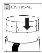
The medium bowl will self-locate into the large bowl. The groove on the small bowl must allign with the pip on the medium bowl.
