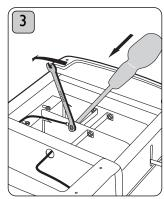
Unscrew brass links and wires.
