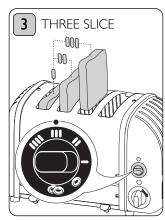
4 slot model: Rotate the 'selector switch' clockwise to the three slice indicator. The first three slots from the left will toast on both sides.
