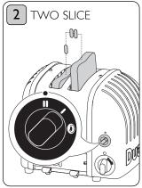
2 & 4 slot models: Rotate to the two slice indicator. The first two slots from the left will toast on both sides.
