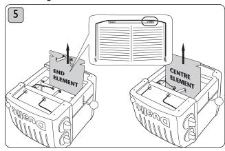
Remove element. To reassemble, reverse procedure ensuring wires and parts are correctly positioned. Ensure new element is marked the same as the one removed. The element heats on both sides and can be inserted facing either way. Check it is seated correctly in the channels either side. Portable Appliance Tested before use.
