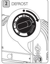
Rotate the 'timer' to the defrost symbol and let the timer wind down to '0'.
