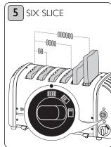
**6 slot model:** Rotate the 'selector switch' clockwise to the six slice indicator. All slots will heat up.
