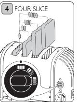
4 & 6 slot model: Rotate the 'selector switch' clockwise to the four slice indicator. The four slots from the left will toast on both sides.
