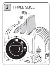
3 slot model: Rotate the 'selector switch' clockwise to the three slice indicator. The three slots from the left will toast on both sides.
