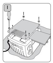
Unplug and place toaster on a soft cloth. Remove crumb tray and unscrew feet to remove the base plate.
