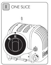
**2, 3 & 4 slot models:** Rotate the 'selector switch' clockwise to the one slice indicator. The left hand slot will heat up on both sides.
