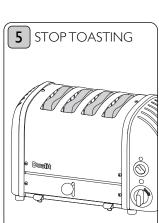
The 'timer' will dick off to 'O' position. To cancel toasting manually rotate the 'timer' to 'O'. If neon light remains illuminated after use immediately unplug the toaster & call service centre.
