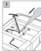
Unscrew brass links and wires.
