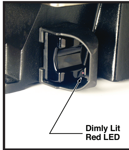
Figure 4-5 Right Operate Switch in Standby Mode, One LED Dimly Lit
