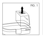
Remove the Upper Motor Housing from the Reservoir Base, being careful not to let the power cord drop into the base (Fig. 2).
