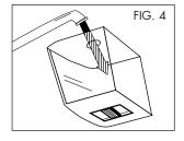
Replace the fill cap by turning it clockwise. DO NOT OVER TIGHTEN.
