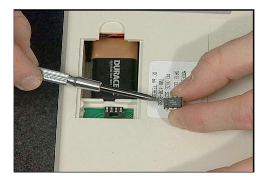
Be careful that the notch is on the correct side of the socket. Check that each pin will slip into the socket.
