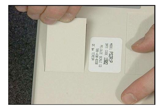
Replace the battery rate chip compartment cover.
