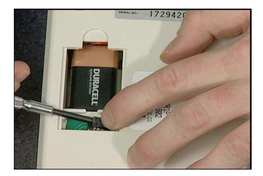
Using a flat head screwdriver gently pry one side up and the other side to remove the chip.
