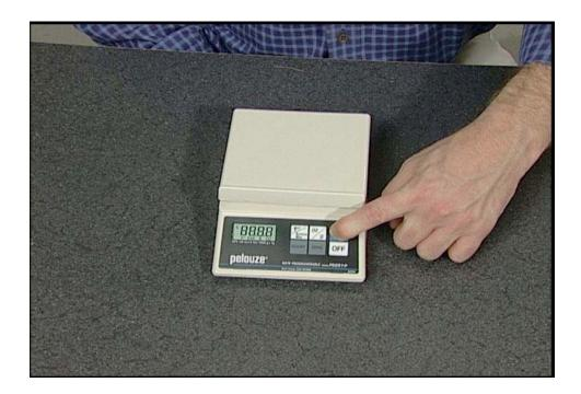
First turn the scale on. The scale must remain on while changing the rate chip to retain the memory.
