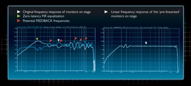
For Dynacord loudspeaker cabinets, measurements of the frequency and phase response are already provided in the IRIS-Net™. This data can be displayed and merged in IRIS-Net™ together with the filter, crossover and delay settings. The superposition then shows the acoustical frequency response of
