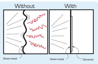
Sheet metal subjected to impact creates noise. With Dynamat installed, the noise is transformed into silent energy through a process called "Vibro-Acoustic Energy Conversion". Dynamat converts the vibrational energy into low-grade thermal energy. The result is a more quiet and comfortable living environment.
