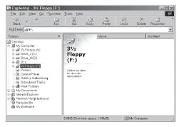
Note: Unlike a general disk drive, the USB FDD is not always assigned the "Drive A" designation. The drive letter assigned depends on your computer's configuration. If there is an internal floppy drive installed on your computer, it will always be assigned as Drive A.
