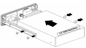
Installing your hard drive in the enclosure 1 Remove two screws on the left side of panel.
