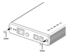
4 Place the hard drive with the plastic cap back into the aluminum housing and secure it with the two screws you previously removed.
