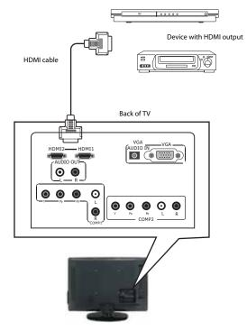
3 Connect the other end of the cable to the HDMI1 or HDMI2 jack on the back of your TV.
