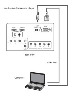
3 Connect an audio cable to the AUDIO OUT jack on the computer, then connect the other end of the cable to the VGA AUDIO IN jack on the back of your TV.
