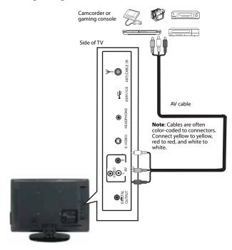
3 Connect the other end of the cable to the AV jack and the AV audio in jacks on the side of your TV.
