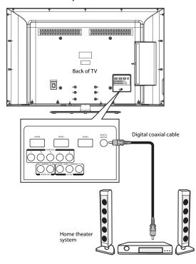
3 Connect the other end of the audio cable to the digital coaxial input jack on the home theater system.
