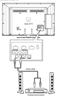
**3** Connect the other end of the audio cable to the input jacks on the analog sound system.
