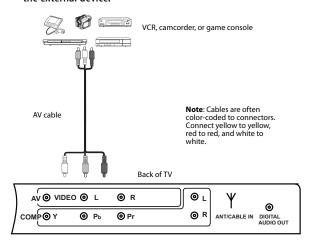
3 Connect the audio connectors of the AV cable (the red and white connectors) to the AV OUT AUDIO jacks of the external device, then connect them to the AV IN1 or AV IN2 L and R jacks on the back of your TV.
