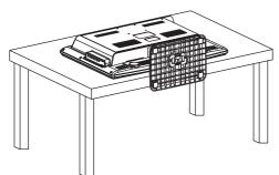
2 Remove the four screws holding the stand column to your TV, then remove the stand column and stand.
