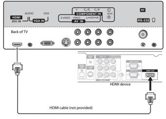
Note: If the external device only has DVI output, use a DVI-to-HDMI adapter cable to connect to the HDMI jack. If you use this configuration, you also need to connect an audio cable from the DVI device to the VGA AUDIO IN jack on the back of the TV. 2 Press INPUT. The *Input Source* menu opens. Select HDMI, then press ENTER to confirm. You can also select HDMI input directly by pressing HDMI.
