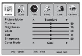
2 Press < or ► to select Lock, then press < . The *Enter Password* screen opens.
