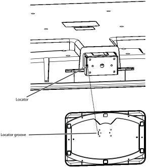
**4** Secure the stand to the column with the four M5 screws (provided).
