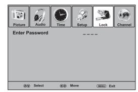
**3** Press the number buttons to enter the four-digit password. The default password is **0000**. You should change the password to a number you can remember. The *Lock* menu opens.
