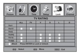
6 Press ▲ ▼ < or ► to select the rating you want to block, then press ENTER. A lock symbol appears when a rating is blocked.</li>
