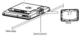
3 Align the holes on the stand with the holes in the stand column and align the locating groove in the stand with the locator in the stand column. Make sure that the locater is fully inserted into the locating groove, or your TV may be unstable and tip over.
