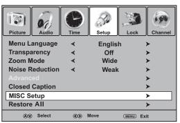
**3** Press  $\blacktriangle$  or  $\checkmark$  to select **MISC Setup**, then press  $\triangleright$  or **ENTER**.
