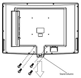
2 Remove the four screws that secure the stand column to your TV, then remove the stand column.
