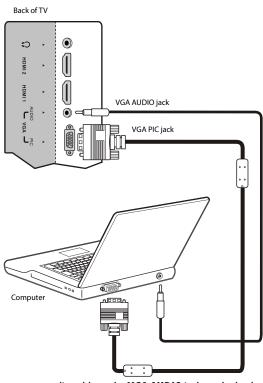
**3** Connect an audio cable to the **VGA AUDIO** jack on the back of your TV, then connect the other end of the cable to the **AUDIO OUT** jack on the computer.
