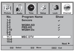
4 Press ▲ or ▼ to highlight the channel you want to delete, then press ENTER to mark the channel. A check mark disappears if the channel is deleted. The check mark appears if you add back the channel.
