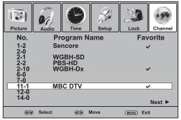
4 Press ▲ or ▼ to highlight the channel you want to add to the favorite list, then press ENTER to mark the channel. A check mark appears if the channel is added to the list. The check mark disappears if you delete the channel from the list.
