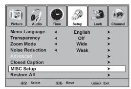
**3** Press  $\blacktriangle$  or  $\checkmark$  to select **MISC Setup**, then press  $\succ$  or **ENTER**.
