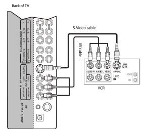
3 Connect the audio plugs on the AV cable to the AV IN AUDIO-L and AUDIO-R jacks on the back of your TV.
