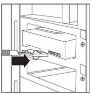
iii. The Serial ATA connectors (4) to any computer components that have a Serial ATA connector, such as a CD/DVD/Blu-ray or hard drive.
