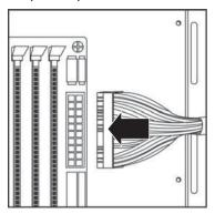
b. Connect the 8-pin (4+4) or 4-pin +12 V power connector to your motherboard.
