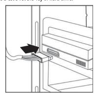
iv. The 8-pin PCI-E or 6-pin PCI-E connector to a PCI-E graphics card.
