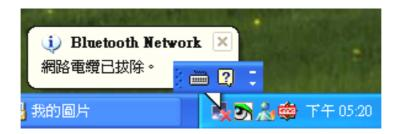
**6.2 Condition 2:** Failure to detect the Bluetooth dongle (The Bluetooth icon turns red, indicating the failure to detect the Bluetooth dongle.)
