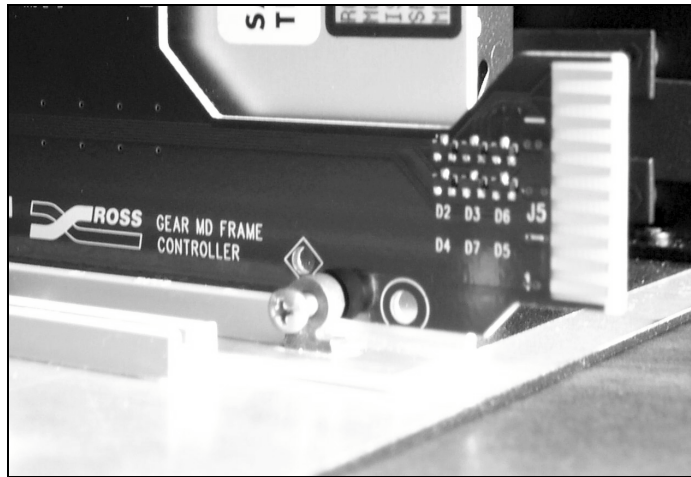
Figure 11. MFC-8310 Fan Controller Card and Unscrewed Retaining Screw
