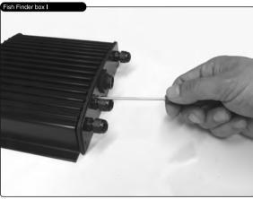
Once the screws are removed, pull out the panel and the Printed Circuit Board (PCB). Unscrew the cables from the PCB.
