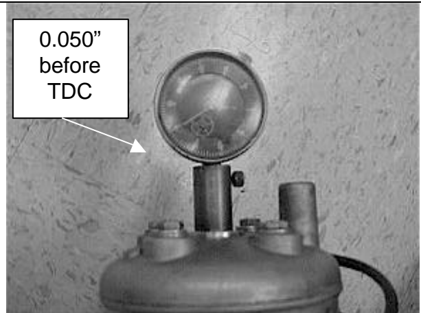
Figure 19, Using a dial indicator to measure piston height for setting ignition timing.
