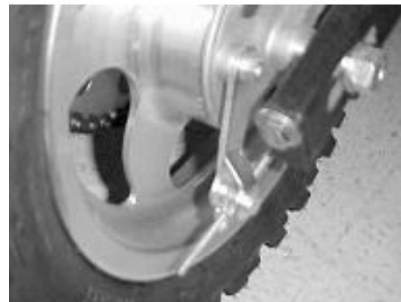
Figure 4, adjust brake lever 'free play'
