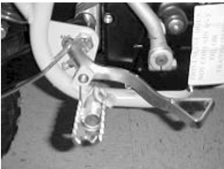
Figure 3, adjust brake lever free height
