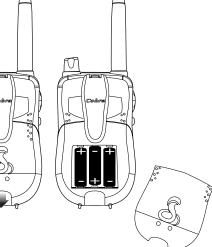
Pull lock tab down to remove battery cover.
