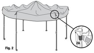
Pull up sliding bracket located on upper portion of leg until push button snaps into place. (Fig. 3) This will ensure upper portion of frame is fully extended.
