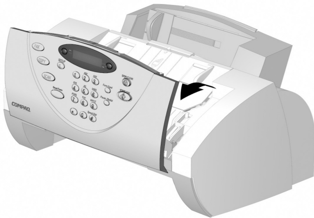
Opening the control panel
