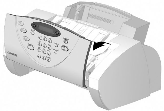
Lifting the control panel
