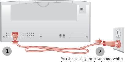
You should plug the power cord, which has a three-wire electrical grounding type plug, into a grounded electrical outlet.
