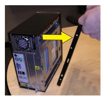
**9** Release the two latching tabs on the left side of the front bezel by pulling them slightly outward. When the left side of the front bezel is released, pull it away from the computer.
