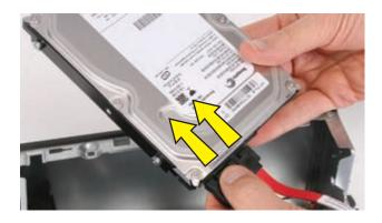
**4** Place the drive so the guide screws fit into the guide screw slots. The drive manufacturer's label should be visible when the drive is in place.
