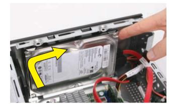
6 Replace the hard drive retention screws and tighten them.
