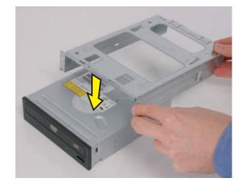
**2** Align the holes marked "2" on the drive cage with the holes on the sides of the disc drive.
