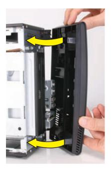
**10** Align the tabs on the inside edge of the left side panel with the slots in the edge of the left side of the computer case.
