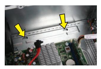
**5** Push the hard drive back into the bay and then to the right until it locks. When the drive is properly located, the threaded holes in the drive line up with the holes in the drive bay, and the power and data cables will route properly.
