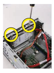
**CAUTION:** Using retention screws that are too long can damage some hard disk drives. The hard disk drive retention screws are slightly shorter than the rest of the screws. Set these screws aside for use with the replacement hard disk drive.
