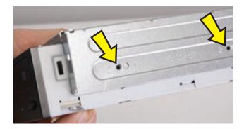
**3** Replace the four drive cage screws.
