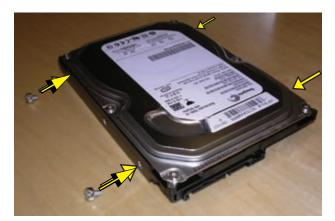
When you hold the drive with the label (A) facing up and the data and power connectors (B) toward you, the guide screws (C) will be to your left when properly installed.
