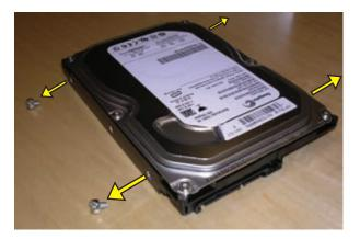
2 Install the guide screws into the new hard drive.
