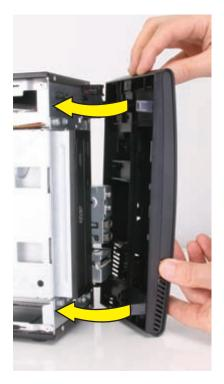
Align the tabs on the inside edge of the left side panel with the slots in the edge of the left side of the computer case.
