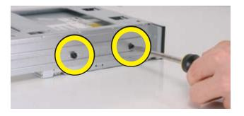
**NOTE:** The black, optical drive cage retention screws are metric screws.
