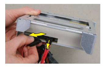
**14** Remove the four screws (two on each side) that hold the optical drive in the drive cage.
