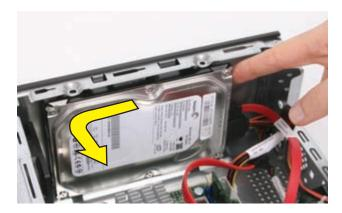
17 Lift the hard drive straight up and out.
