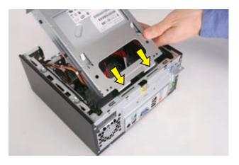
9 Replace the two optical drive cage screws.
