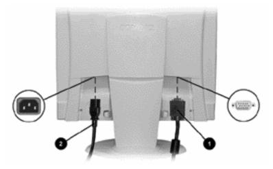
3. Connect one end of the AC power cord (2) to the monitor and the other end to an electrical outlet that is easily accessible and close to the monitor.
