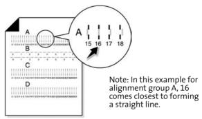
Using the same **up**, **down** and **start/yes** buttons used in step 4, change the value for the letter displayed on the printer LCD, and then press **start/yes** to select it. The next alignment letter will be shown until you have set all the alignment values for the page.
