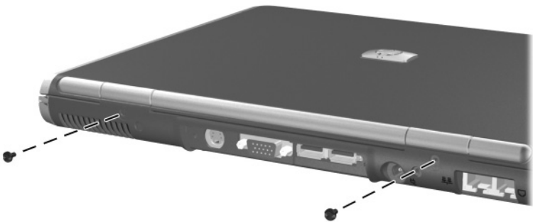
Removing the Display Assembly Screws
