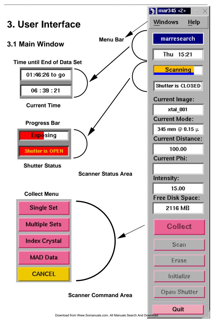
The main window controls the most important scanner functions. It consists of different areas:
