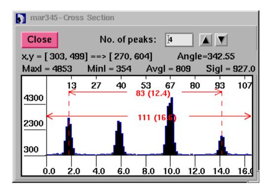
This window is used for displaying cross sections through the image. The window can be obtained by pressing the left mouse button in the image area.
