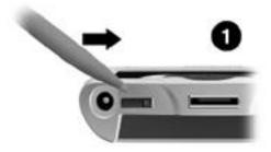
2. Slide the On /Off switch to the Off position using the stylus. Wait about one minute, then slide the switch to the On position.
