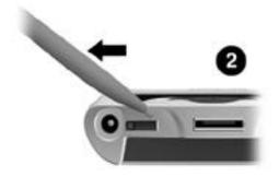
3. Close the Battery On/Off door using the stylus.
