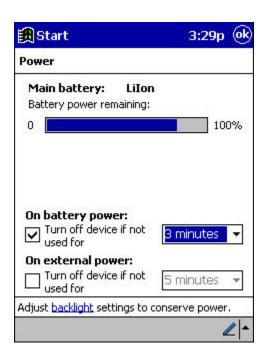
The Power control panel only shows the battery charge level if you are using the battery. If you have connected the AC adapter, the window shows the recharging status.
