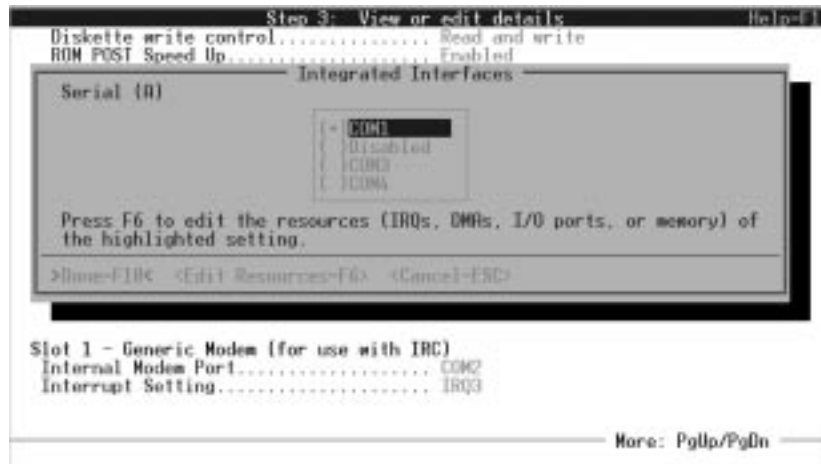
Figure 2-3. Example: Configuring an integrated serial port
