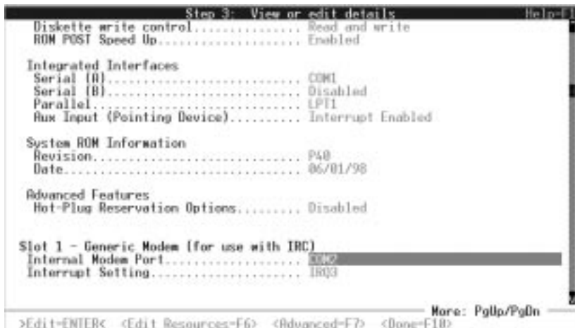
Figure 2-2. Example: Setting the COM and IRQ resources
