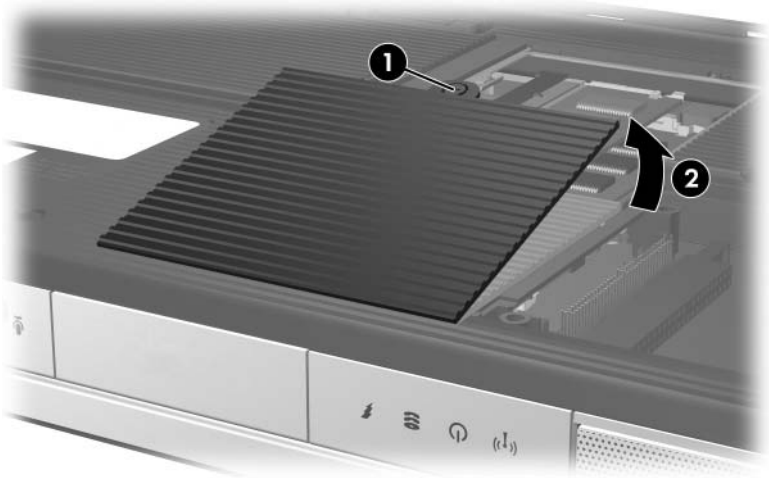
Removing the Mini Card Compartment Cover
