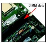
There are two memory module slots on the system board for installing main memory. You can install 266MHz DDR-SDRAM modules, these are available in 128, 256 and 512MB memory modules. You can install a maximum of 1GB (2 x 512MB modules).
