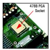
The Compaq Evo D310 Micro Desktop is equipped with either a socket 478B Intel Celeron or Pentium 4 processor. The processor is connected to the system board through a Pin Grid Array (PGA) 478B Socket.
