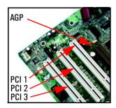
The Compaq Evo D310 Micro Desktop has four accessory board slots: three PCI slots and one 1.5V AGP slot.
