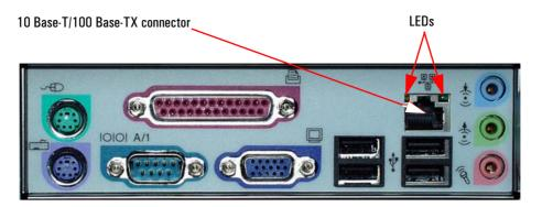
There are two LEDs on the 10 Base-T/100 Base-TX connector as indicated in the graphic above. The following table provides a status summary of these LEDs:
