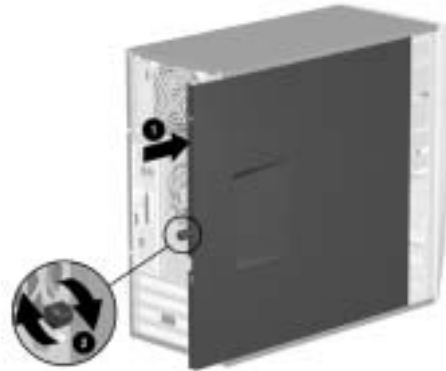
replacing the side access panel on the S0000 series
