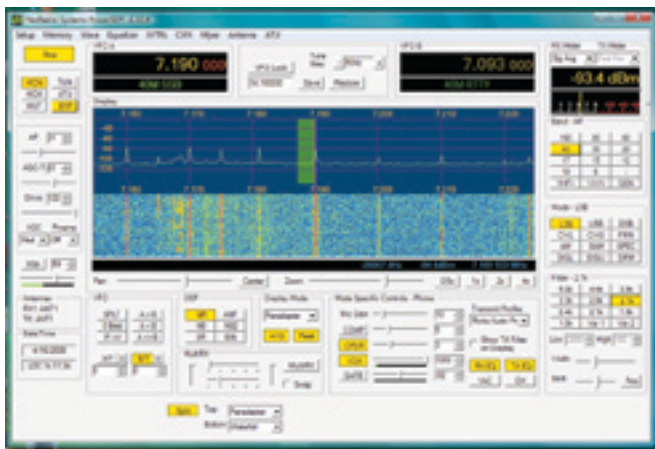
Figure 5 — You can split the PowerSDR screen to show any combination of the panadapter and waterfall displays.
